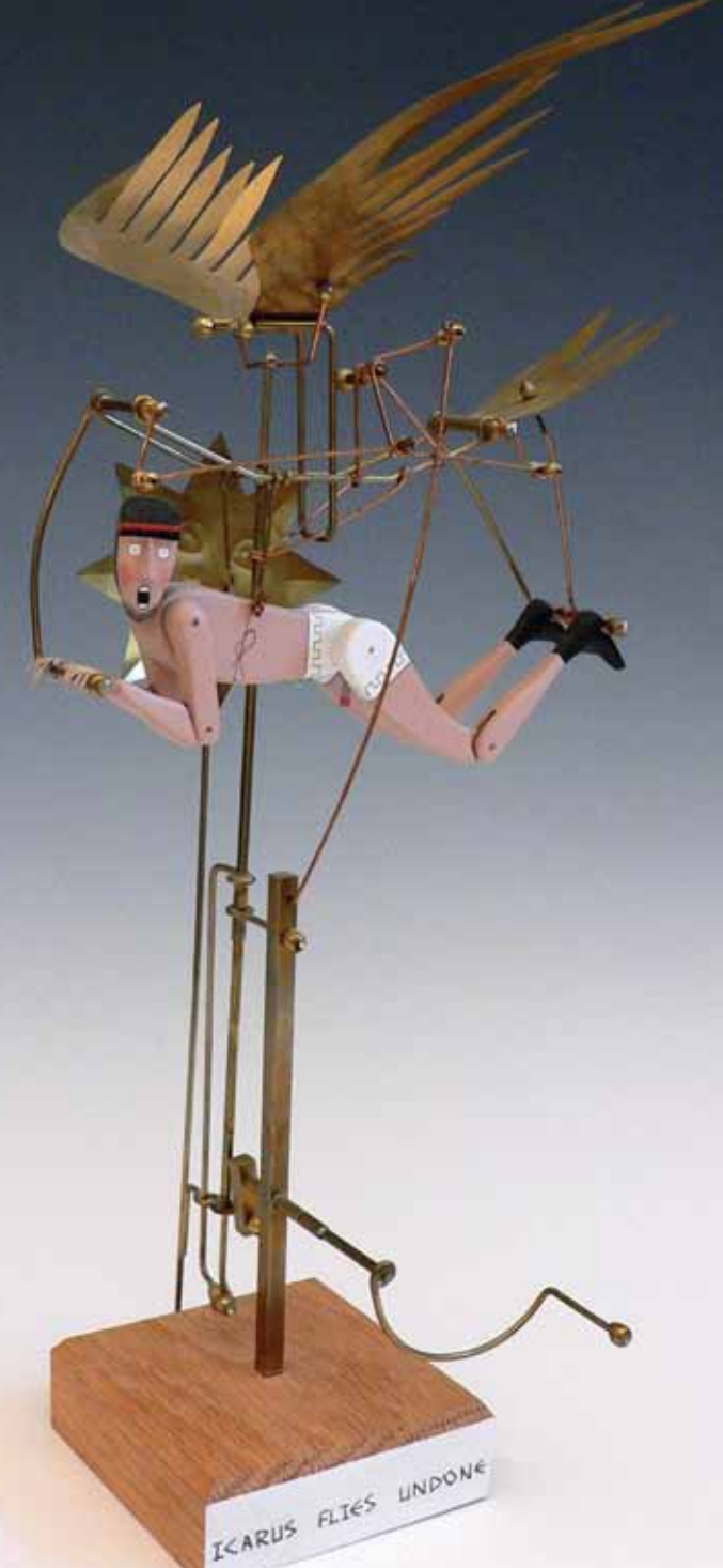
The mechanism is based on a crank slider. Drawing 1 (with the stand in green) shows the back of the base and the bottom of the crank slider, attached to an offset rod which passes, at a 90° angle, through the base pillar to the crank handle C . The primary shaft Sh passes through a piece of brass tube (a bearing mount Bm ) attached to the pillar. This mount can pivot to allow the crank slider to rock back and forth. Drawing 2 shows the “bird cage” from the front. The shaft moves up/down and in a gentle rotary motion, following the motion of the hand crank, and providing the primary movement. Because the wings are fixed to the shaft housing, they are made to “flap” because of the motion of the crank slider. The internal rods, colored red in this drawing, work as a single unit, rotating at the joints. A longer rod Rd is fixed to the base, so that, like the wings, other parts must move to compensate for the action of the crank slider shaft. The Icarus figure’s feet Ft are attached to the back crossbar; his hands Hd are attached to the front one. A tether attaches to the tail “feathers” and waves them up and down. As the crank slider shaft follows the motion of the crank handle, Icarus’ hands and feet alternately pull and push, as if he is “working” the wings.
